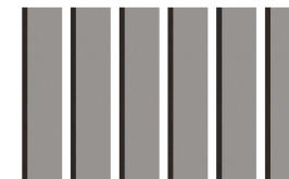
6 Aluminium Balustrades & Screens 75mm Vertical Angles, Dulux Powdercoat - to match glazing frames
